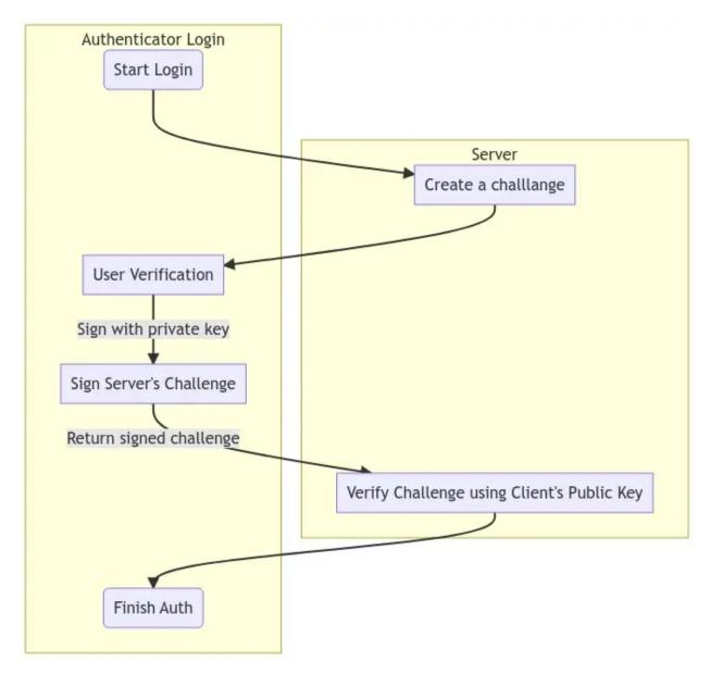
Because of this mechanism, it is impossible to phish WebAuthn credentials, as they are never released from the authenticator. Only the signed challenge is released, which is not enough to obtain the credentials. Because a large portion of cyberattacks come from breached passwords, this can massively improve your security.
